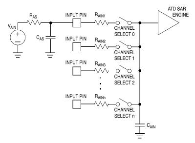
Figure 6. Resistor and Capacitor Placement
