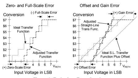
Figure 2. Endpoints Error Graph
