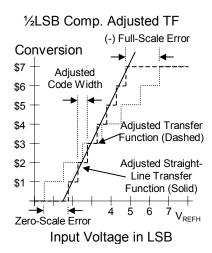
Most ADC's exhibit some non-linearity at the endpoints due to the difficulty in measuring a signal that is identical to the reference. If these errors are accounted for, a more accurate portrayal of the ADC behavior in application is possible. For this reason, the *Adjusted Straight-Line Transfer Function* is drawn between the minimum input voltage plus the *Zero-Scale Error* ( $V_{REFL} + E_{ZS}$ ) to the maximum input voltage plus the *Full-Scale Error* ( $V_{REFH} + E_{FS}$ ).
