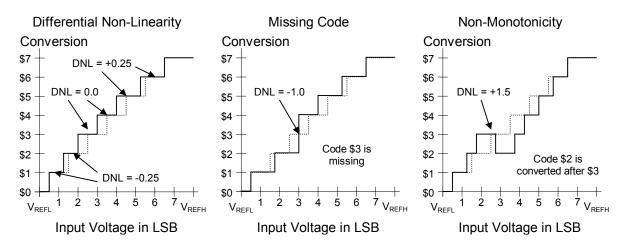
Figure 3. Differential Non-Linearity, Missing Codes, and Non-Monotonicity Graphs
