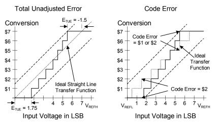
Figure 4. Total Unadjusted and Code Error Graphs
