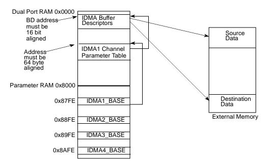
Figure 2. Memory Structure for IDMA Operation
