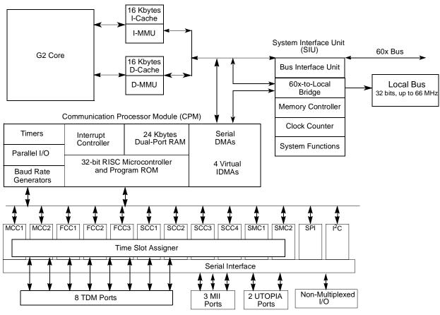
Figure 1. MPC8260 Block Diagram
