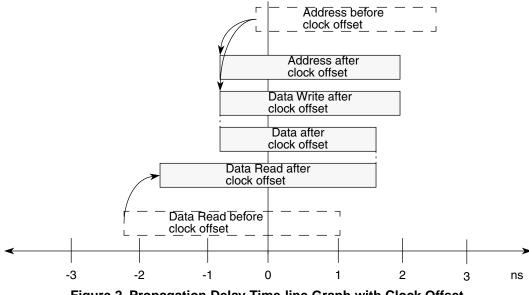
Figure 2. Propagation Delay Time-line Graph with Clock Offset
