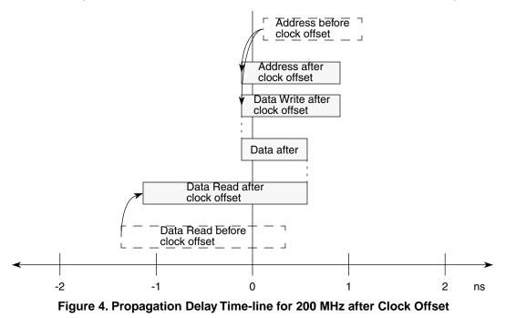
Notice the real trade-off has been a decrease in address propagation time for an increase in data propagation time and an increase in both the address and data hold time margin. For this example, the data overlap increased 2x the clock offset, while the address decreased only 1x the clock offset.
