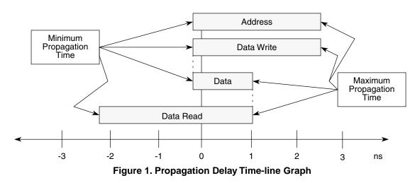
Once the ranges are plotted, they can be analyzed to determine if there is a need to shift the ranges by using clock offsets. As shown in Figure 1, the left side of a range represents the minimum propagation delay while the right side represents the maximum propagation delay for that cycle type. Notice the data signal group has two cycle types—data write and data read. The actual range allowed for a data signal is the overlap of the data write and data read ranges.
