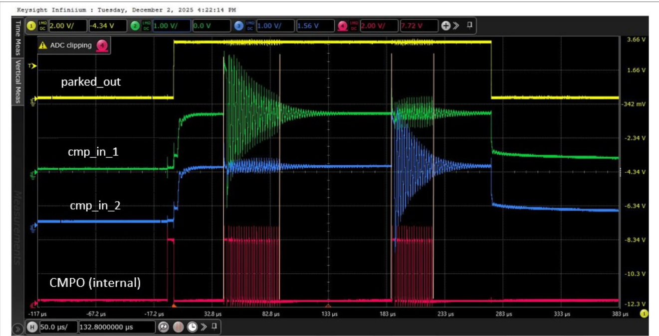
Figure 23. Two-LC sensor oscilloscope traces with comparator output
