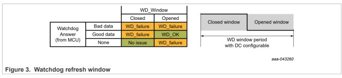
For FS6500 and FS4500 ASIL B version, the watchdog is simple and refreshed by the MCU using any key. The only requirement is the watchdog refresh time must in the second half (open window) of the whole watchdog window. It is suggested to make the watchdog refresh at 3/4 of the watchdog window.
