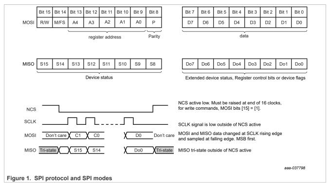
When configuring the SPI protocol in the MCU driver or in the configuration tool, configure it as:
