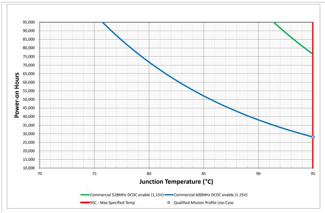
Figure 1. i.MX RT1040 commercial lifetime estimates for DCDC-enabled mode
