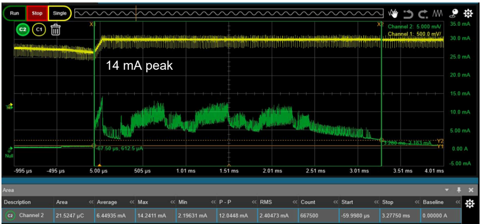
Figure 8. DC-DC Ramp control enabled and DCDC_RAMP_CNTRL = 5
