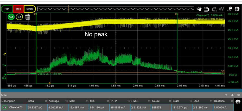
Figure 12. DC-DC Ramp control enabled and DCDC_RAMP_CNTRL = 1
