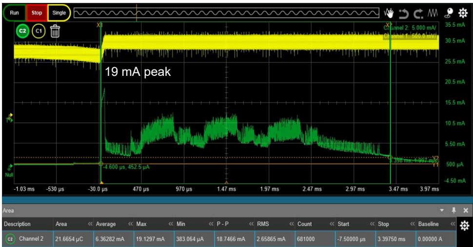
Figure 6. DC-DC Ramp control enabled and DCDC_RAMP_CNTRL = 7
