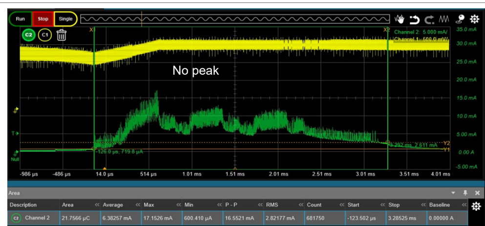
Figure 11. DC-DC Ramp control enabled and DCDC_RAMP_CNTRL = 2
