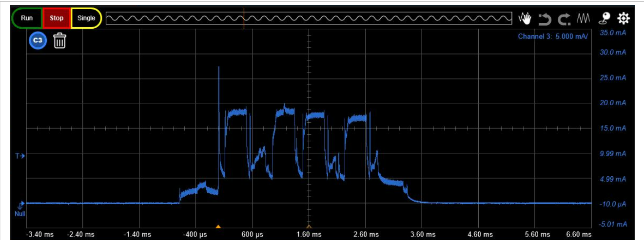
Figure 38. Advertising current profile, +10 dBm, no scan response, Bypass mode
