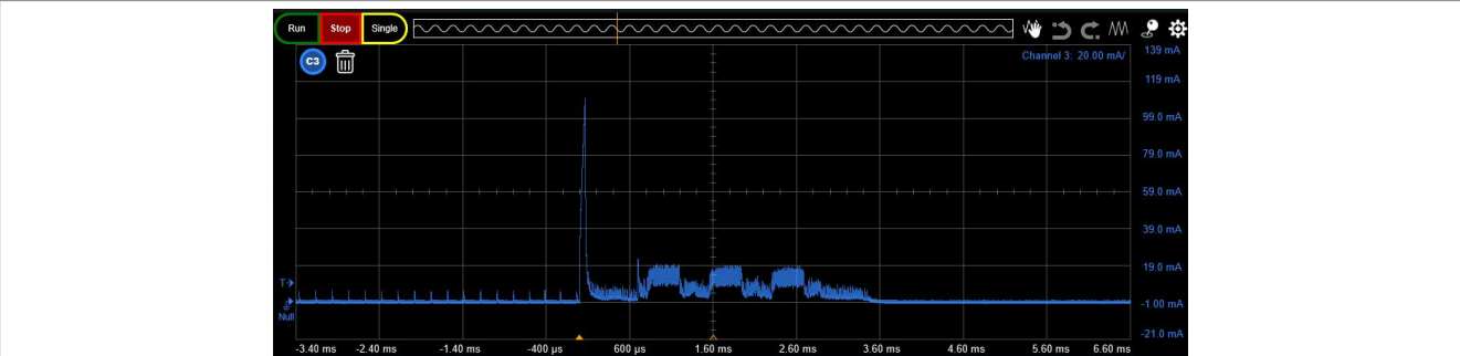
Figure 29. Advertising current profile, +10 dBm, no scan response, Buck mode
