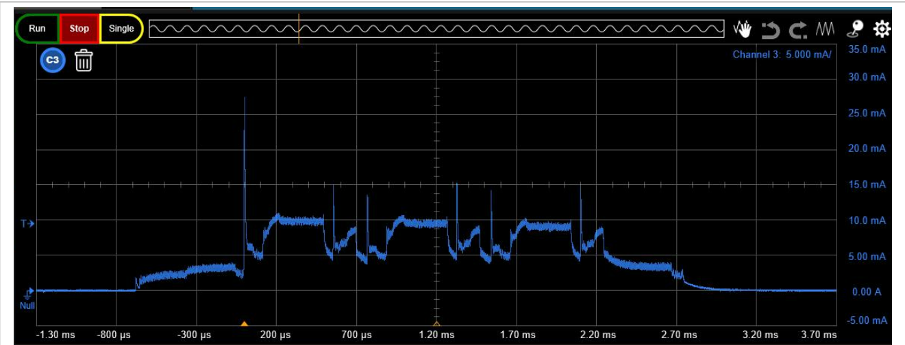
Figure 34. Advertising current profile, +0 dBm, no scan response, Bypass mode
