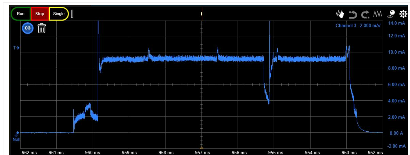
Figure 68. Scan current profile, DCDC_out = 1.25 V, Bypass mode
