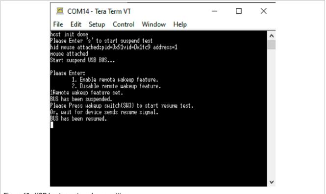
Figure 13. USB host remote wake-up setting
