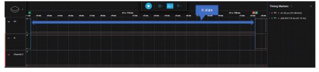
Figure 11. USB FS USB remote wake-up timing
