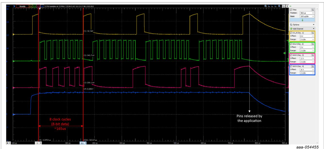
Figure 12. SPI signals during the transfer implemented in the demo project
