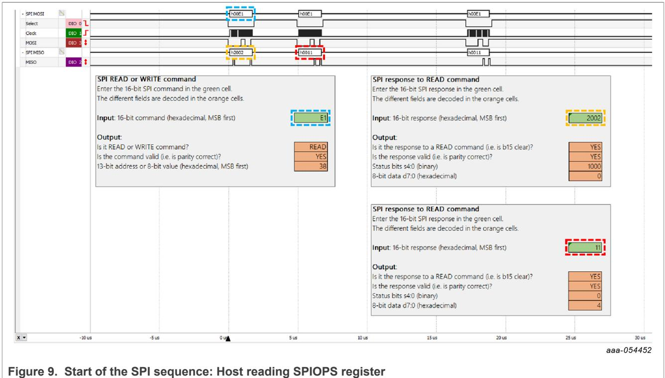
Figure 9. Start of the SPI sequence: Host reading SPIOPS register
