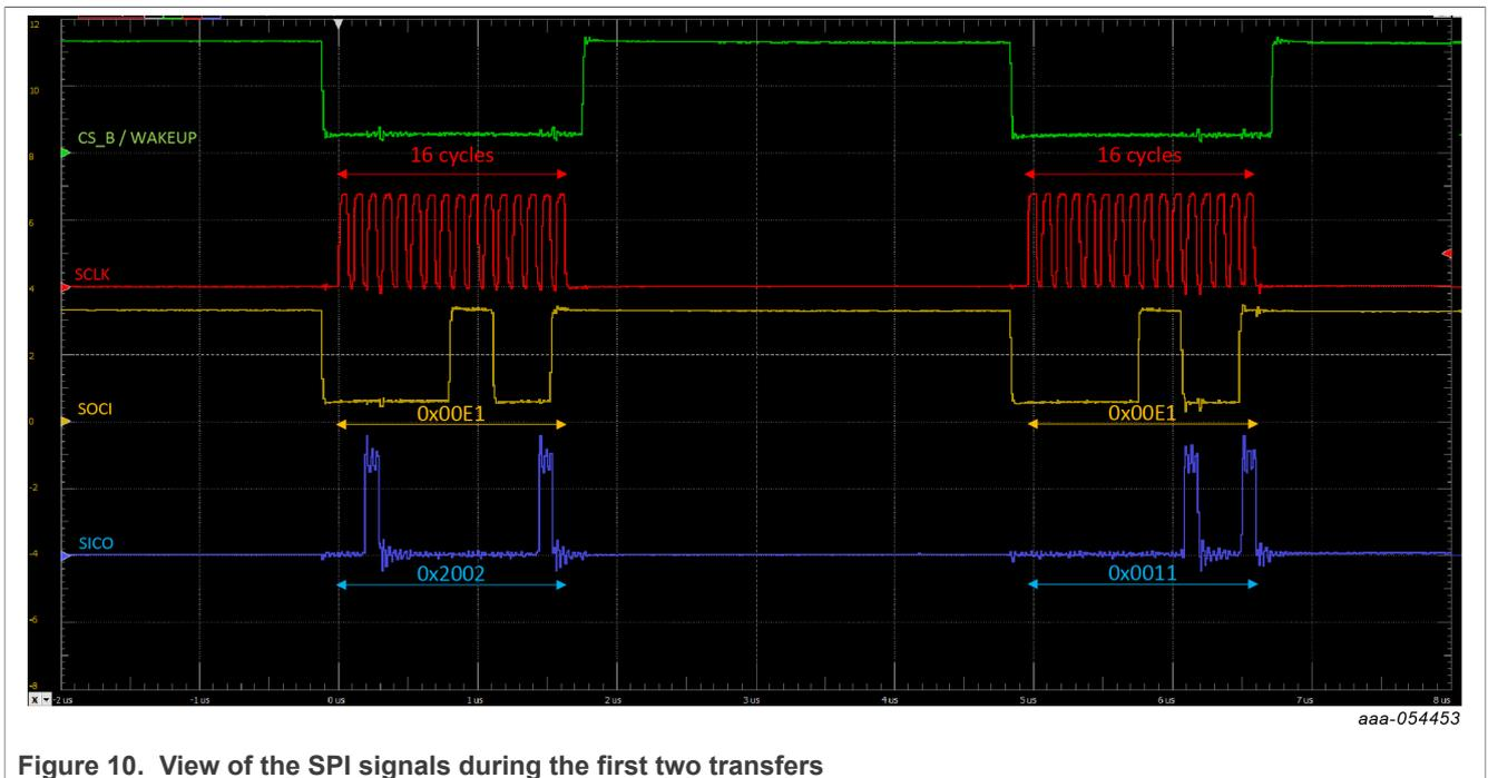
Figure 10. View of the SPI signals during the first two transfers
