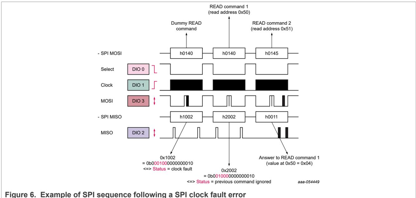
Figure 6. Example of SPI sequence following a SPI clock fault error
