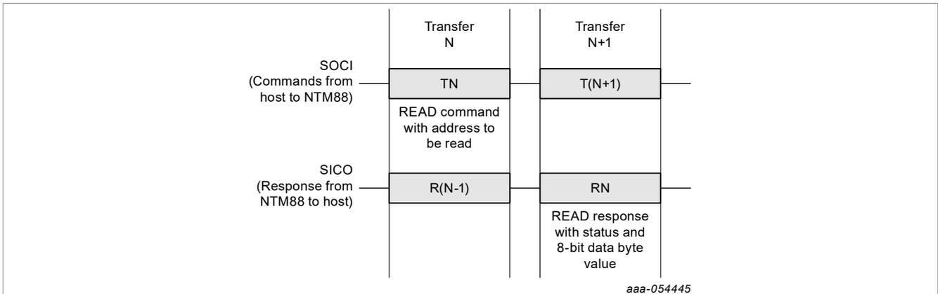
Figure 2. Transfers for a READ operation
