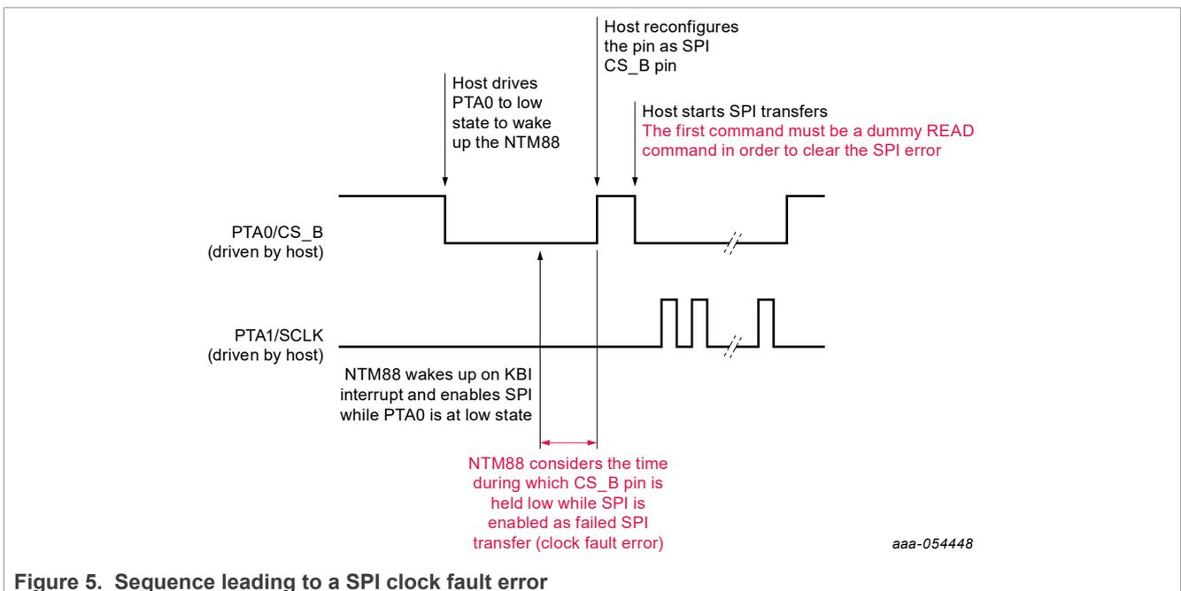
Figure 5. Sequence leading to a SPI clock fault error
