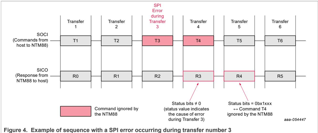
Figure 4. Example of sequence with a SPI error occurring during transfer number 3
