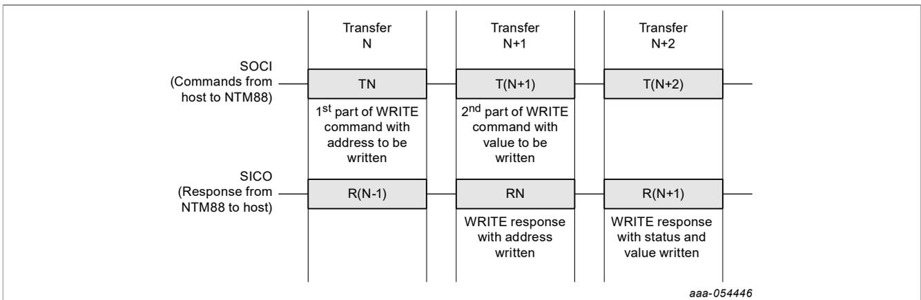
Figure 3. Transfers for a WRITE operation
