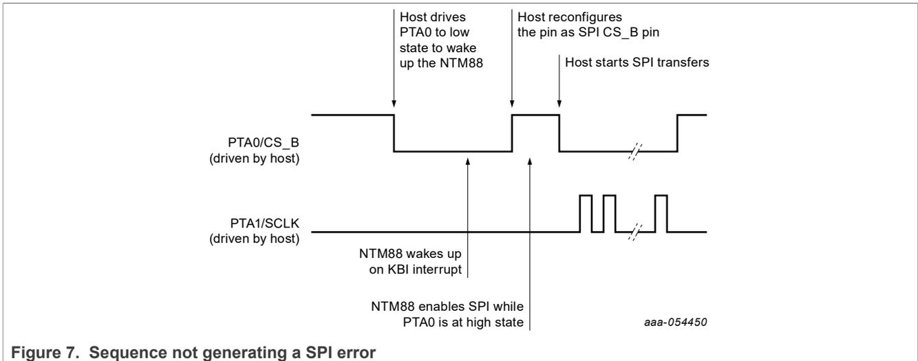
Figure 7. Sequence not generating a SPI error
