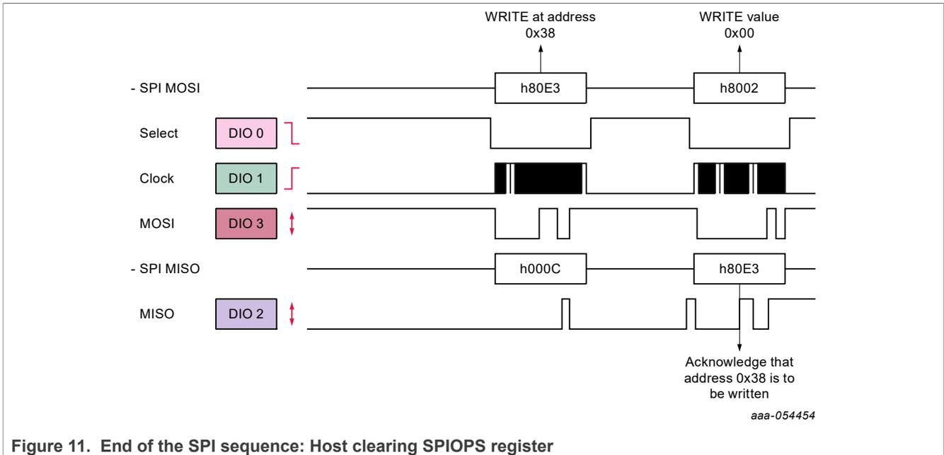
Figure 11. End of the SPI sequence: Host clearing SPIOPS register
