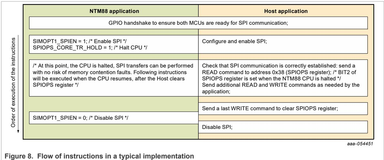
Figure 8. Flow of instructions in a typical implementation
