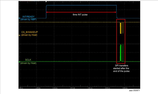
Figure 7. Signals during an NBP8 transfer request
