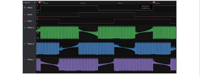
Figure 11. Hall signal and motor-winding terminal at 1000 rpm
