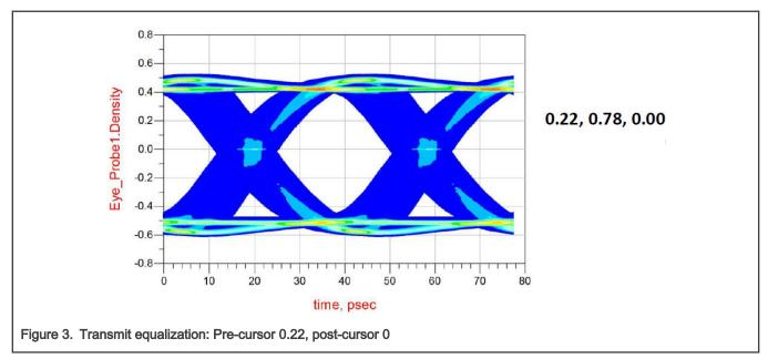
In Figure 3, the pre-cursor is adjusted to 0.22 (1.67x or 4.4 dB), resulting in an increased eye opening.
