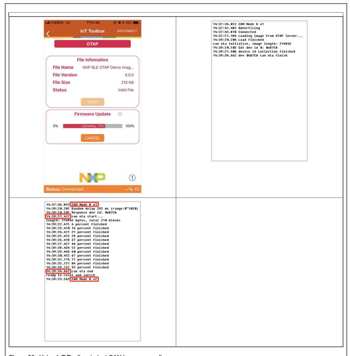
Figure 38. Using IoT Toolbox to test CAN image upgrading
