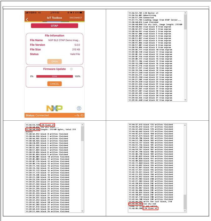
Figure 37. Using IoT Toolbox to test LIN image upgrading
