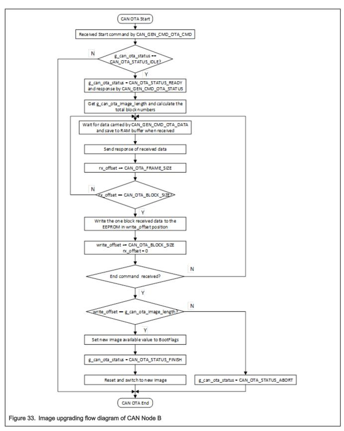
The CAN baud rate is up to 1 Mbps. To consider the stability of upgrading process and support multi-nodes upgrading, you need to upgrade the nodes one by one if there are multiple identical Node B in the same bus. All Node B have different device identifiers.
