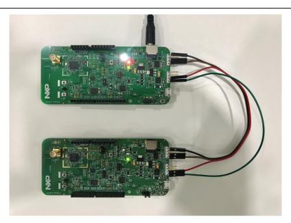
Figure 1. Using FRDM-KW36 DK boards to debug LIN/CAN communication
