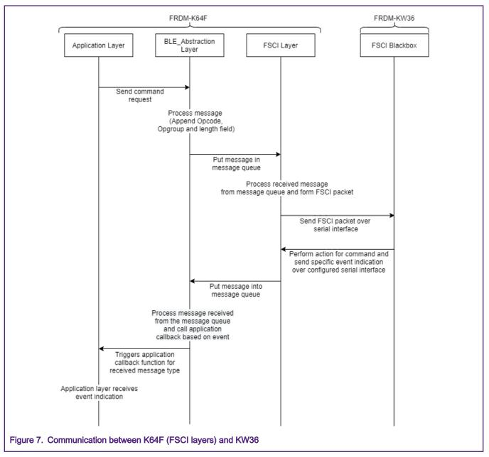
• FRDM-K64F application has three layers: Application layer, Bluetooth LE Abstraction layer, and FSCI layer.
