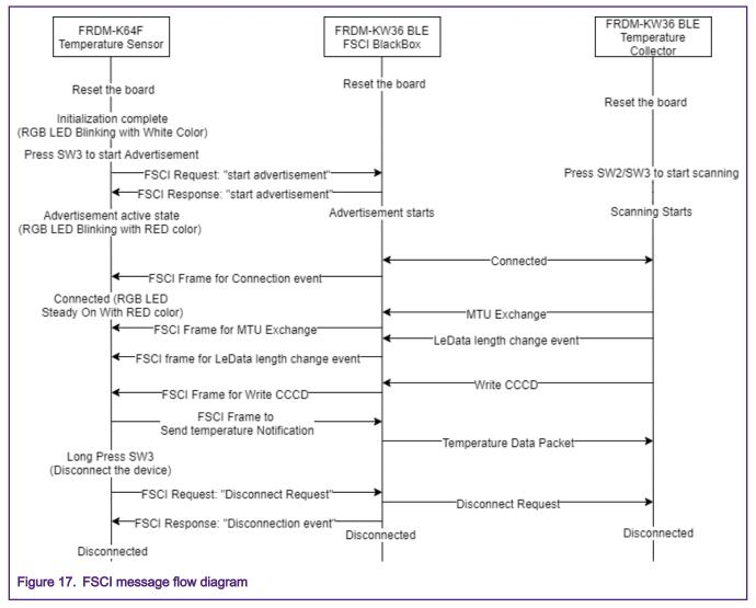
When both devices are connected, the temperature sensor application system is ready to send temperature data as described in Temperature value sending mechanism. The above figure shows the message flow between the boards.
