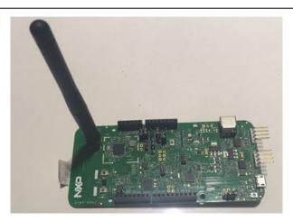
Figure 12. FRDM-KW36 board with monopole antenna
