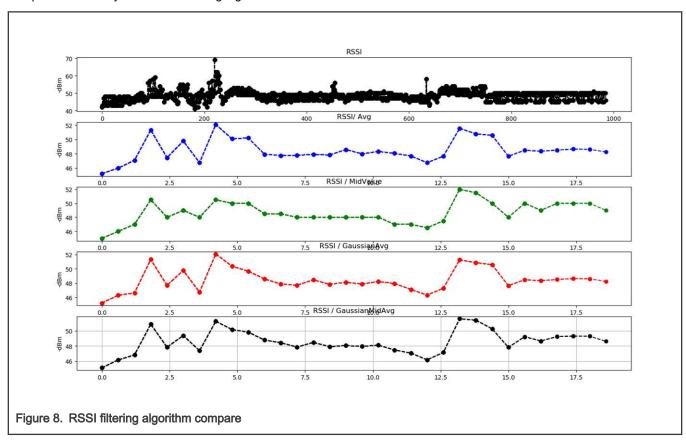
In the test shown in Figure 8, the Tag and Anchor devices are placed in a fixed position. The Anchor device collects and filters the RSSI. The first row is the RSSI measurement and the other rows are the optimized RSSI values of the filtered output. In Figure 8, all filtering has 30 samples with a stepper window of n=30.
