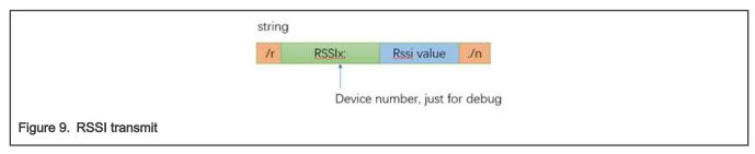
For example, if the RSSI value that the KW36 must transmit is -40 dbm, then it prints the "/ rRSSI: -40./n" string from the UART port.
