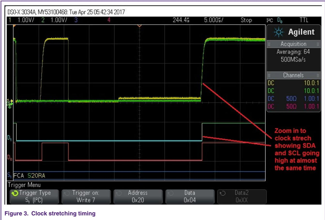
**Figure 3. Clock stretching timing**
