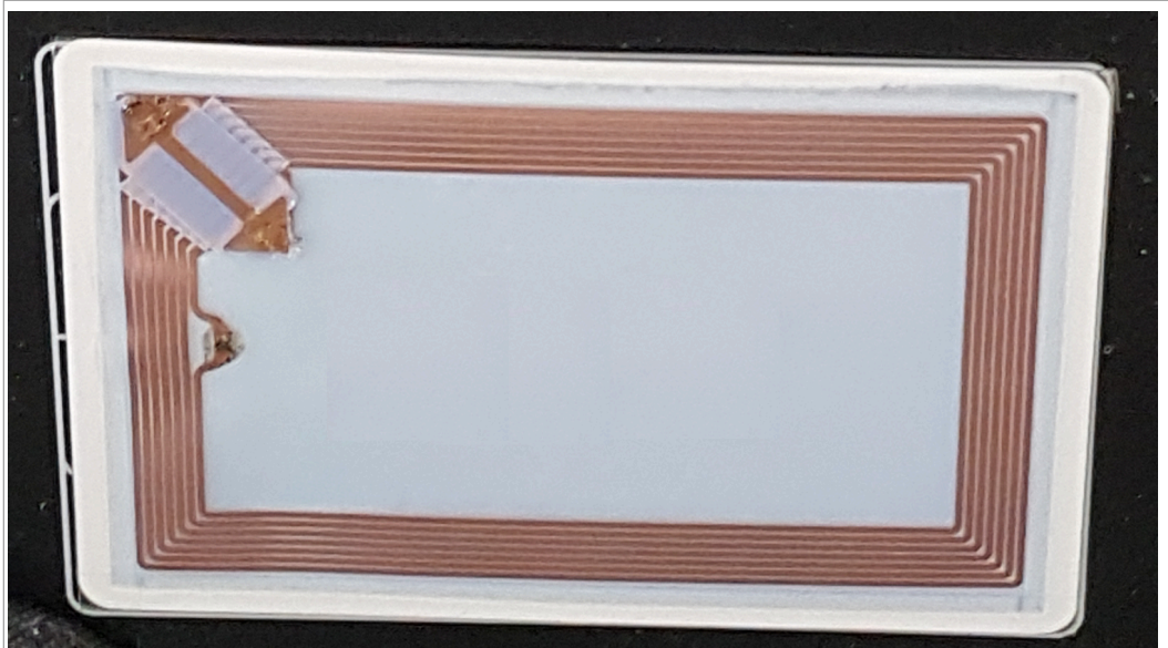
Figure 5. Class 1 Etched Antenna example - Prototype
