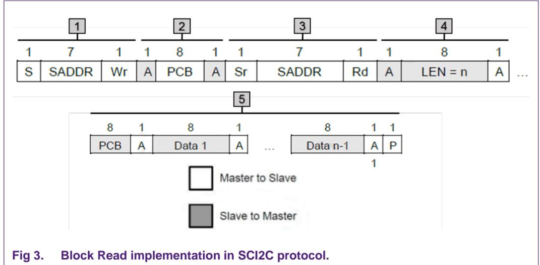
Fig 3. Block Read implementation in SCI2C protocol.
