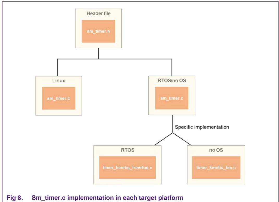
Fig 8. Sm\_timer.c implementation in each target platform
