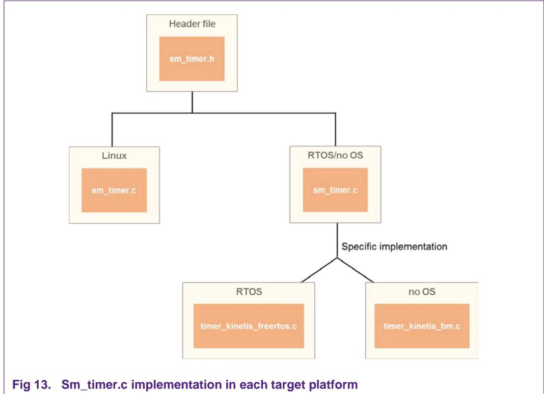
The A71CH Host Library provides the ‘sm\_timer.c’ file already adapted for the Kinetis family. Fig 14 shows the implementation of the ‘sm\_usleep()’ function for this case. As can be observed, the sleep time is defined by the macro CORRECTION\_TOLERANCE. This macro depends on the Compiler used and the core clock frequency of the Kinetis MCU used (FRDM\_KW41Z, FRDM\_K82F or FRDM\_K64F).
