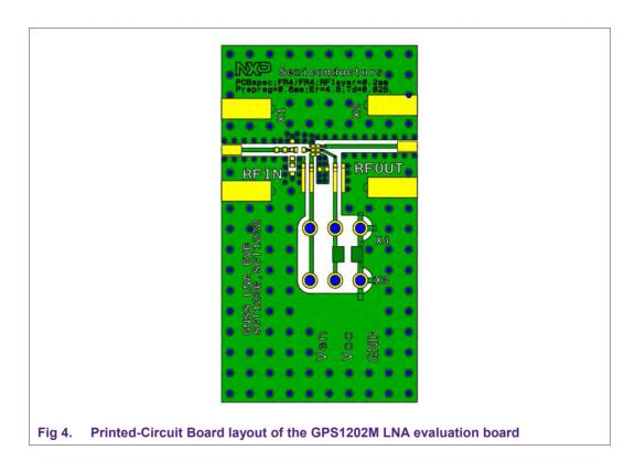
The material that has been used for the evaluation board is FR4 using the stack shown in Fig 5.
