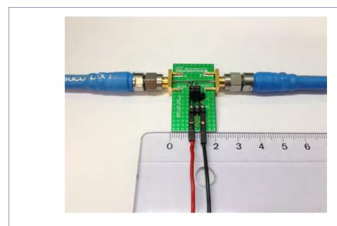
Fig 13. Evaluation board including its connections
