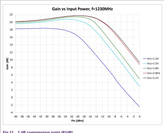
Fig 11. 1 dB compression point (P1dB)
