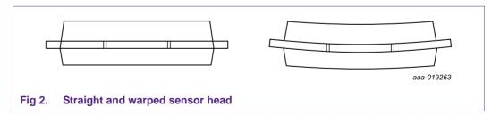
Often the sensor is attached to a substrate (e.g. a throttle body cover). The sensor should be decoupled as much as possible from the substrate, e.g. by using a soft silicone glue to fix the sensor.
