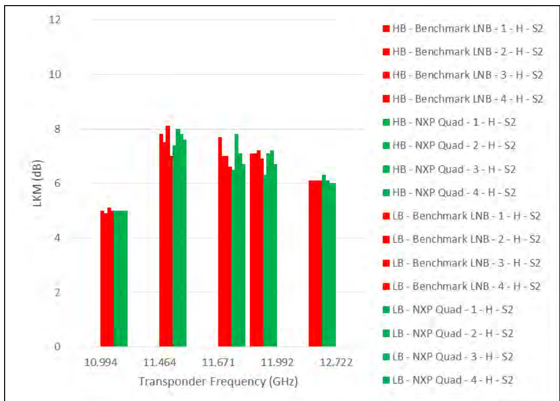
Figure 43 LKM in live signal receiving at horizontal polarity The LKM of NXP Quad and the Benchmark LNB are comparable
