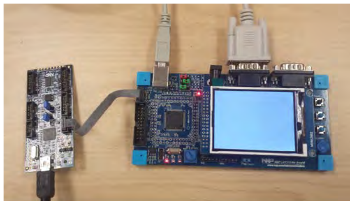
Fig 11. UART and debugger connection on LPC11U68 Manley Board
