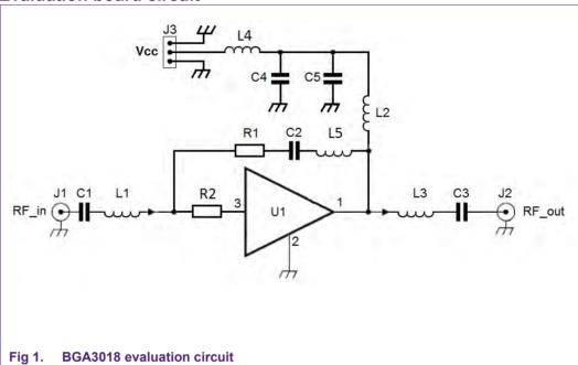
The power supply is applied on the center pin of connector J3 and is applied to the MMIC via choke L4 and L2 which provides RF blocking to the supply line. Capacitors C4 and C5 are supply decoupling capacitors.
