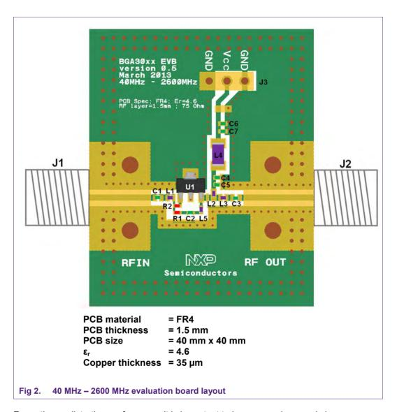
For optimum distortion performance it is important to have enough ground vias underneath and around the MMICs ground pins. This lowers the inductance to the ground plane. The evaluation board is made with two layer FR4 material.
