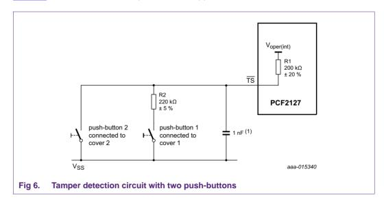
Figure 6 shows the double tamper detection application.
