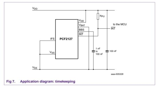
If CLKOUT is enabled during time keeping as described in sections 5.6 to 5.10, the best accuracy is achieved if a CLKOUT frequency other than the default value of 32.768 kHz is selected.
