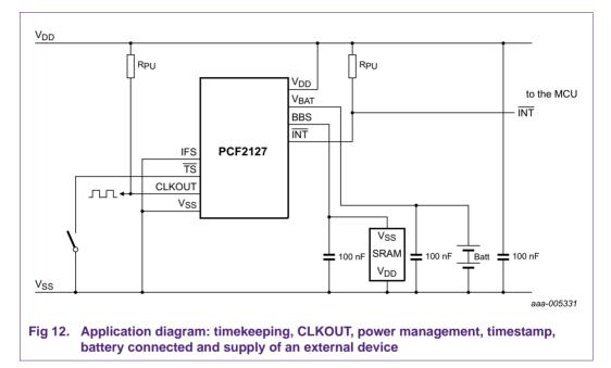
For using the PCF2127 for timekeeping, power management, CLKOUT with a battery connected and supplying a microcontroller, see Figure 13:
