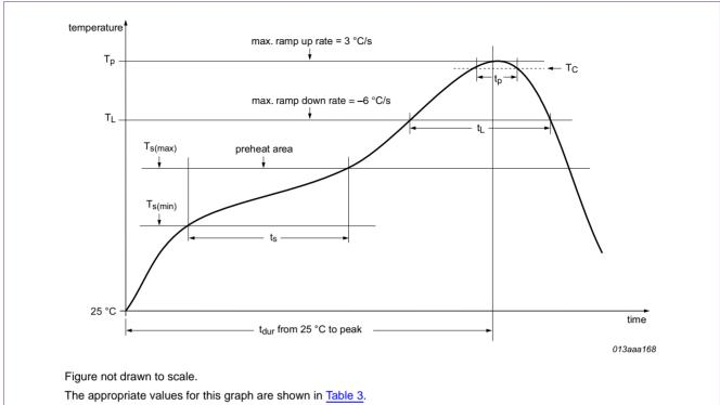
**Remark:** The reflow profile in this document is for classification/preconditioning and not meant to specify board assembly profiles. Actual board assembly profiles should be developed based on specific process needs and board designs, but must not exceed the parameters shown in <u>Table 3</u>.
