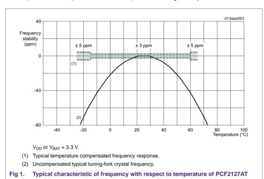
Figure 1 and Figure 2 show the typical frequency stability of the PCF2127 with respect to the temperature in comparison to an uncompensated tuning fork crystal.
