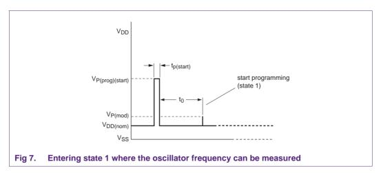
The frequency  $f_o$  can either be monitored directly at pin RESET or as a modulation of the supply current (a modulating resistor of 30 k $\Omega$  is connected between V<sub>DD</sub> and V<sub>SS</sub> when the signal at pin RESET is HIGH, increasing the supply current accordingly).
