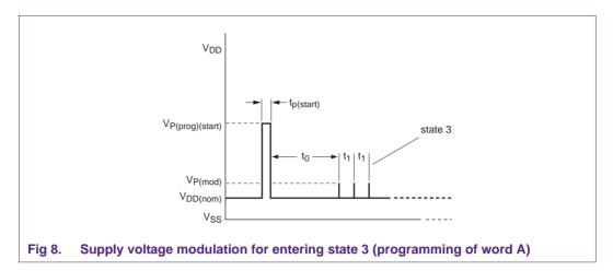
After state 3 has been entered the programming of the word and leaving state 3 is as indicated in the example of Figure 8.
