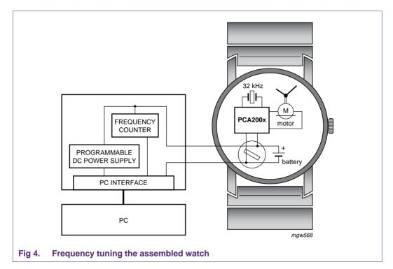
Executing a power-on-reset, writing to the OTP cells and performing the related functional checks is achieved in the PCA200x by modulating the supply voltage. The necessary control circuit consists basically of a voltage level detector, an instruction counter which determines the function to be performed and an 8-bit shift register, which allows programming the OTP cells of an 8-bit word in one step and which acts also as a data pointer for checking the OTP content.
