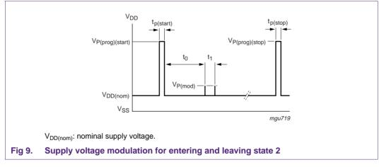
Figure 9 above indicates how to enter and leave state 2. Figure 10 below indicates the output waveforms that appear at pin RESET in state 2.
