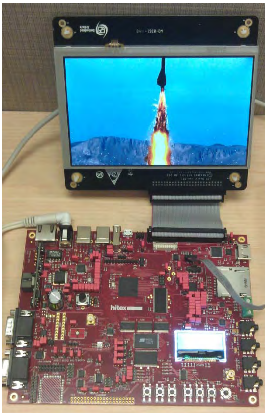
Fig 1. LPC1857 board from Hitex
