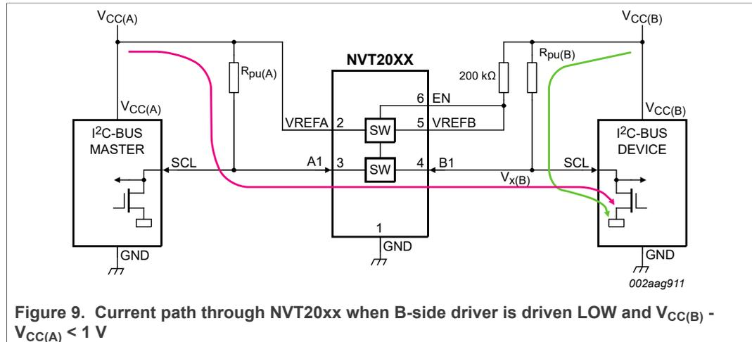
Figure 9. Current path through NVT20xx when B-side driver is driven LOW and  $V_{CC(B)} - V_{CC(A)} < 1\text{ V}$
