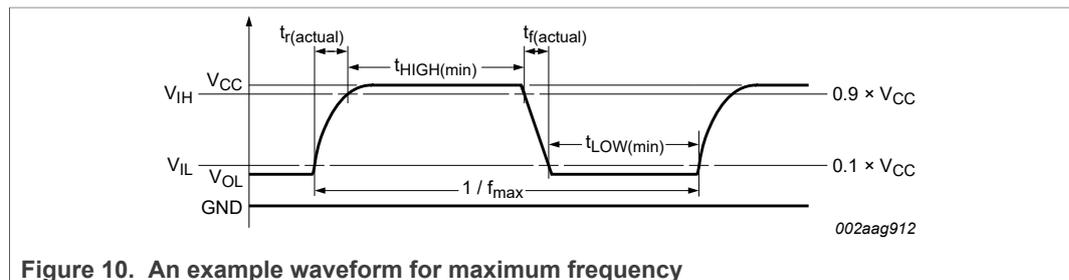
Figure 10. An example waveform for maximum frequency
