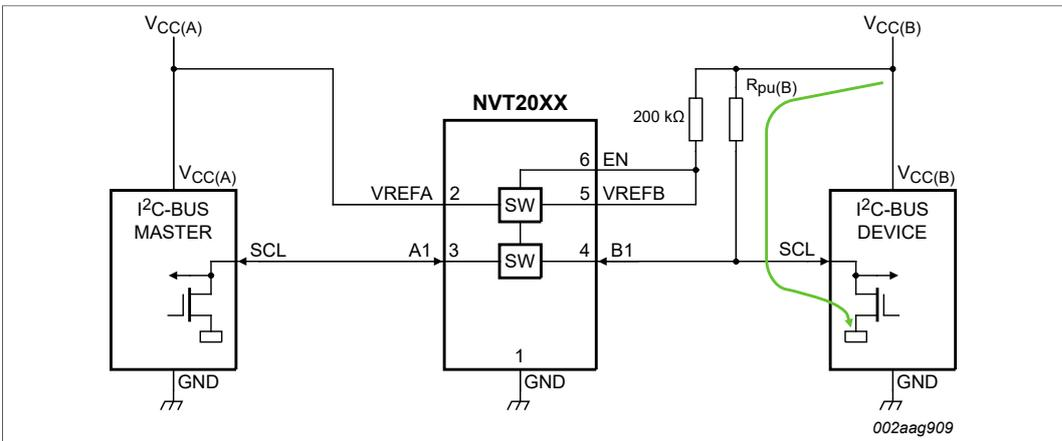
Figure 7. Current path through NVT20xx when B-side driver is turned on and  $V_{CC(B)} - V_{CC(A)} \geq 1V$
