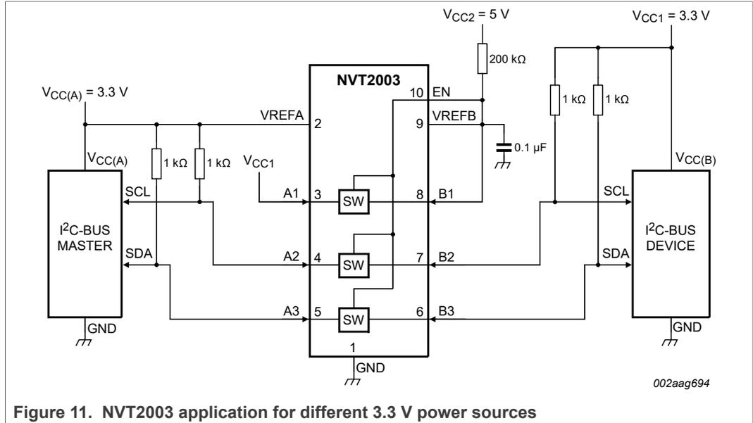
Figure 11. NVT2003 application for different 3.3 V power sources
