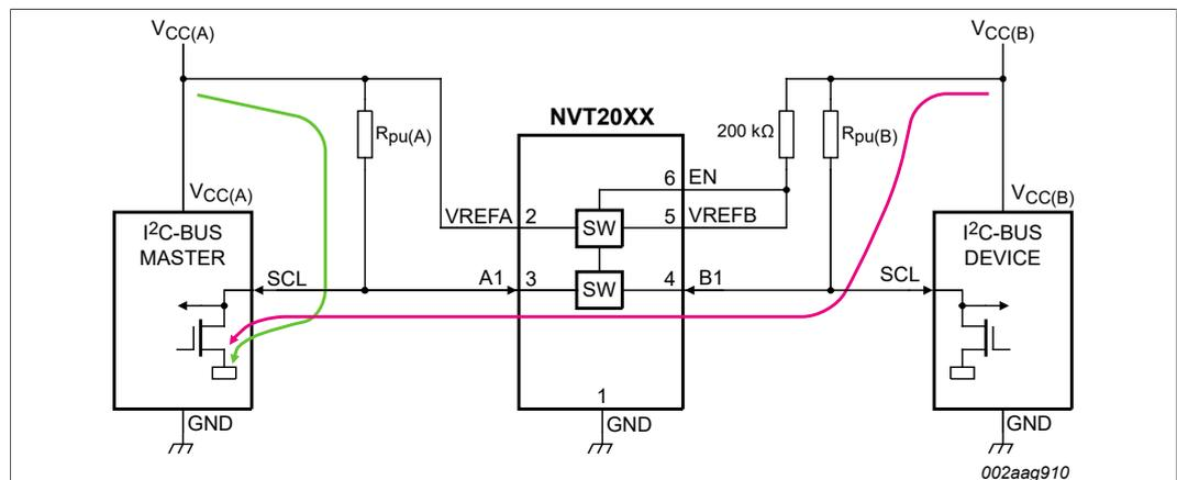
Figure 8. Current path through NVT20xx when A-side driver is driven LOW and  $V_{CC(B)} - V_{CC(A)} < 1\text{ V}$
