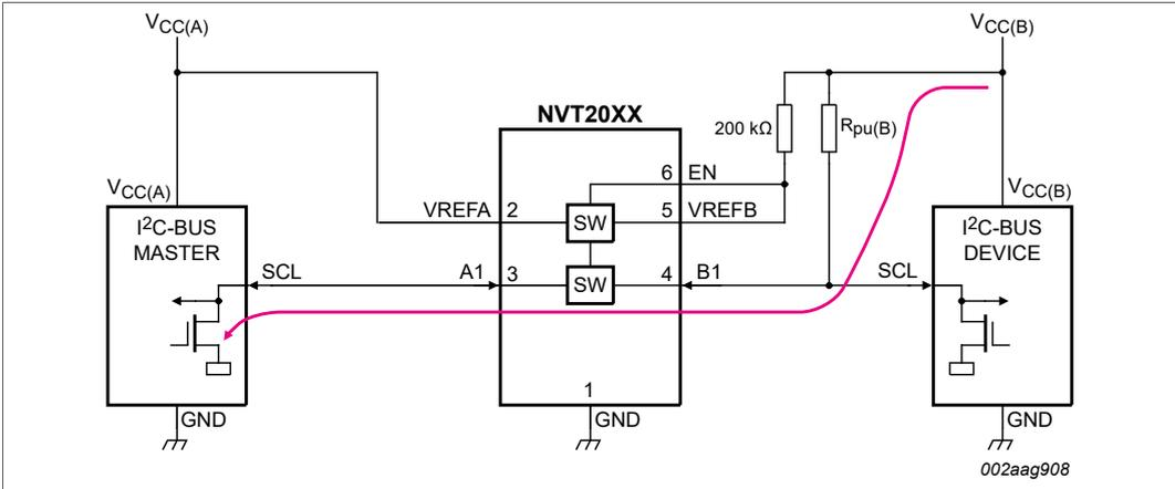
Figure 6. Current path through NVT20xx when A-side driver is turned on and  $V_{CC(B)} - V_{CC(A)} \geq 1V$
