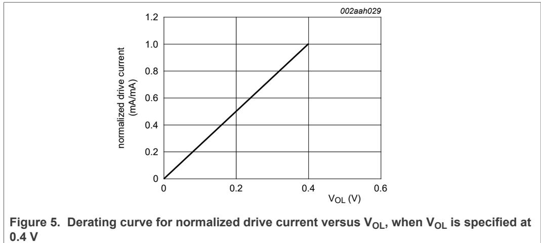
If the specified V<sub>OL</sub> is lower than the required V<sub>IL</sub>, then it is safe to use the specified I<sub>OL</sub> current without any modifications. When using the calculations found in this document, it is assumed that either V<sub>OL</sub> is lower than V<sub>IL</sub>, or that the drive current strength has been derated for a lower V<sub>OL</sub>.
