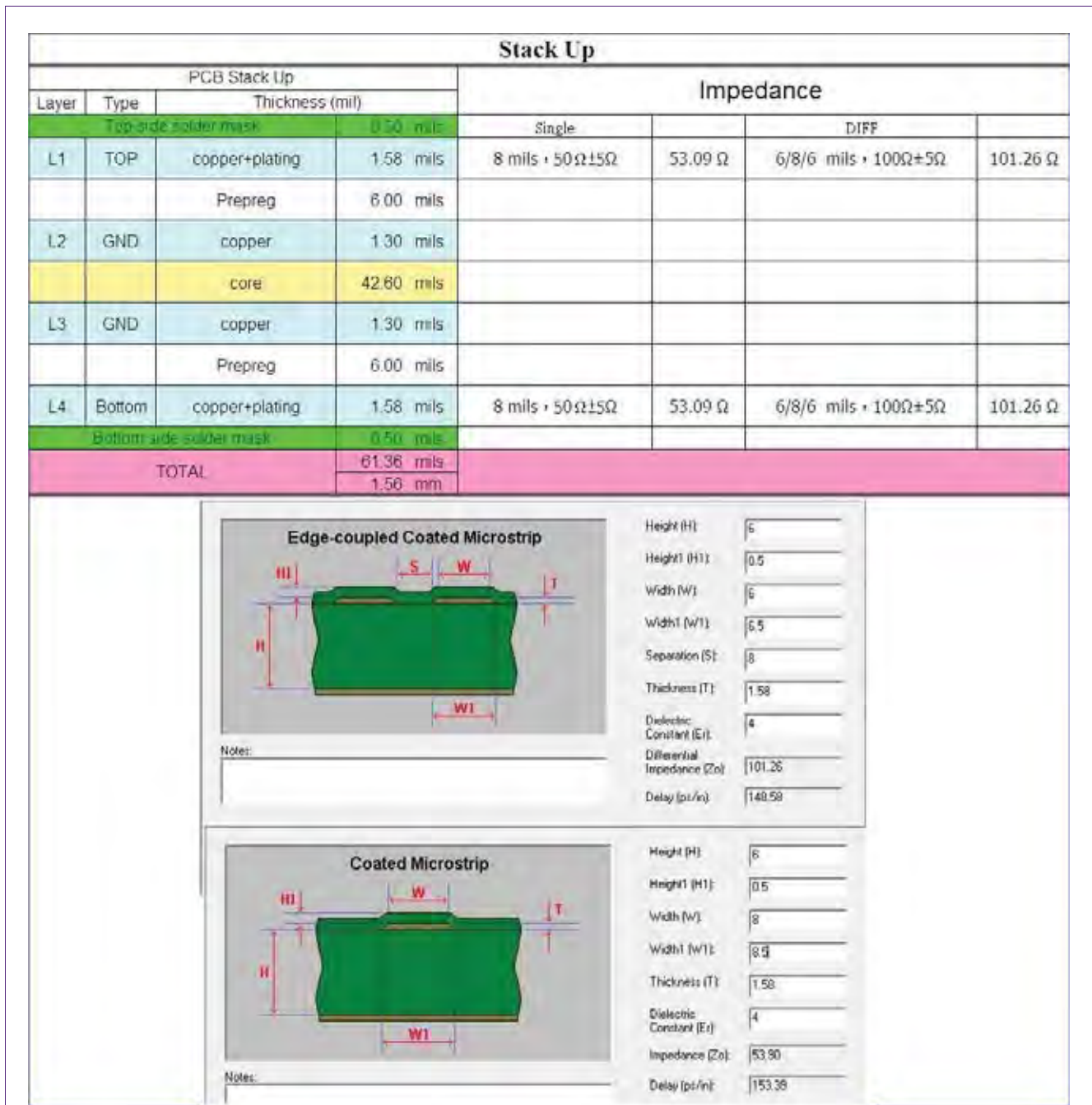
Fig 2. DP-LVDS PCB stack-up example
