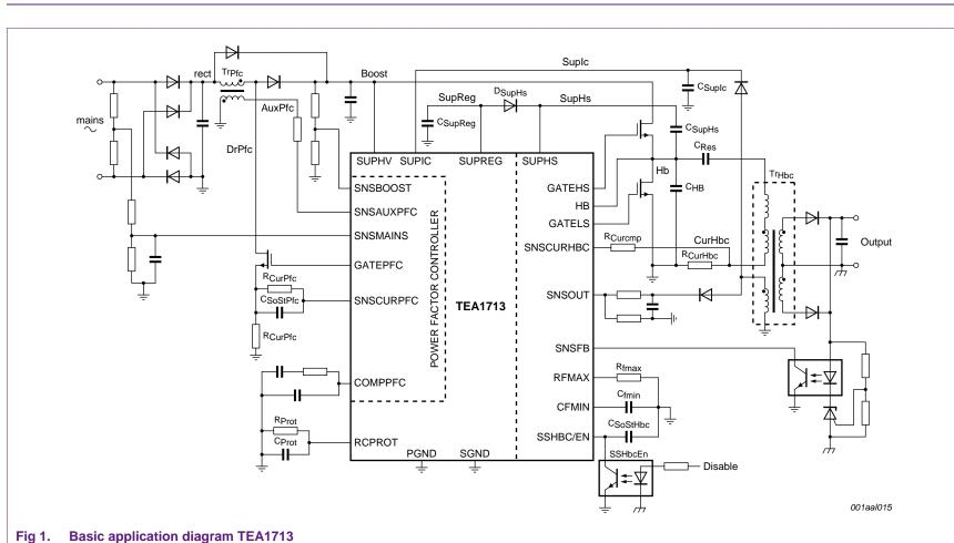
TEA1713 resonant power supply control IC with PFC
