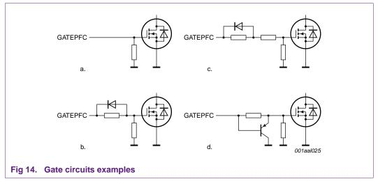
Switching the MOSFETs on and off by the drivers can be approximated by alternating charge and discharge of a (gate-source) capacitance of the MOSFET through a resistor (R<sub>DSon</sub> of the internal driver MOSFET).
