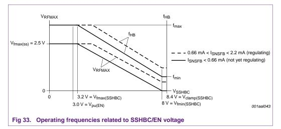
At start-up, the SSHBC/EN voltage is low which corresponds to the maximum frequency. During the soft-start procedure, the external capacitor is charged, the SSHBC/EN voltage rises and the frequency decreases. The contribution of the soft-start function ends when SSHBC/EN is above 8 V.
