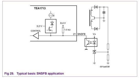
The SNSFB pin supplies the OPTO coupler from an internal voltage source of 8.4 V via an internal series resistor of 1.5 k $\Omega$ . This internal series resistance allows spike filtering by an external capacitor at the pin if needed.
