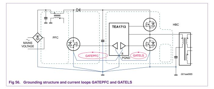
TEA1713 resonant power supply control IC with PFC
