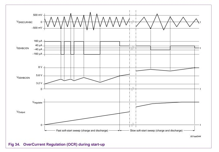
The slow (dis)charge speed is used for the lower frequency range where VSSHBC/EN is above 5.6 V. In the lower frequency range the current in the converter reacts strongly to frequency variations.
