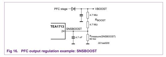
The boost output voltage value is set with a resistor divider between the PFC output voltage and pin SNSBOOST. When in regulation, the SNSBOOST voltage is kept at 2.5 V.
