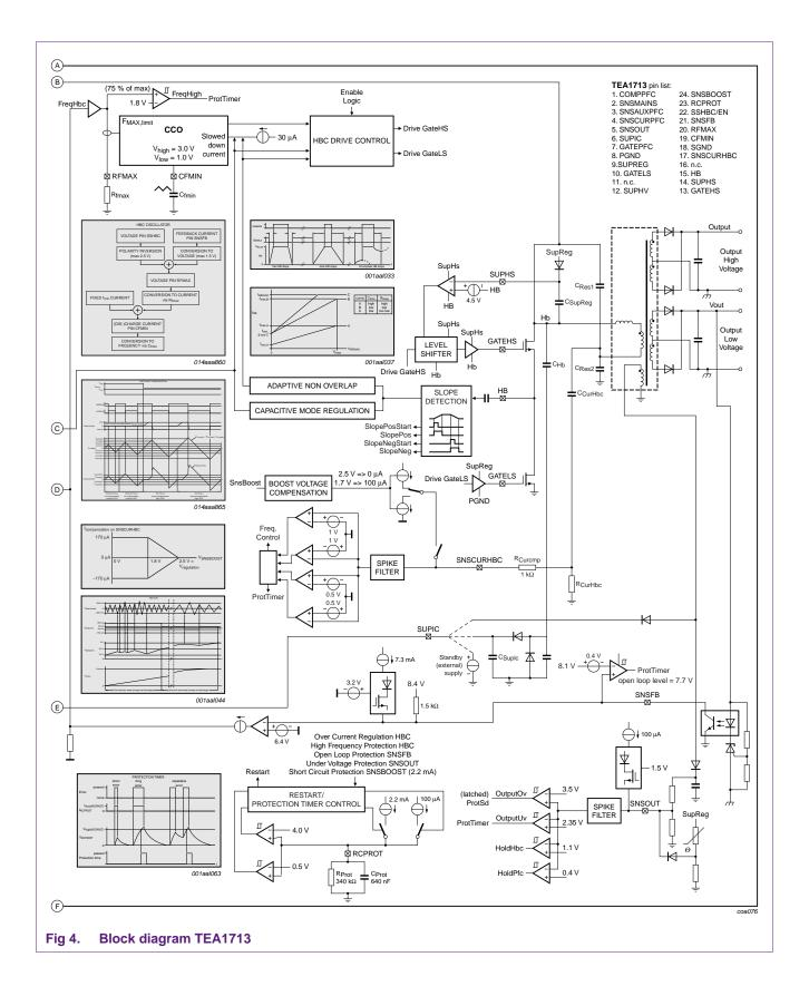
TEA1713 resonant power supply control IC with PFC
