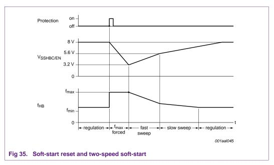
The soft-start reset is also used to ensure a safe start-up at maximum frequency when the HBC is enabled by SSHBC/EN or after a restart. The soft-start reset is not used when the operation has been stopped for Burst mode.
