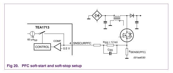
A resistor and a capacitor between SNSCURPFC and the current sense resistor  $R_{SENSE(PFC)}$  set both functions.
