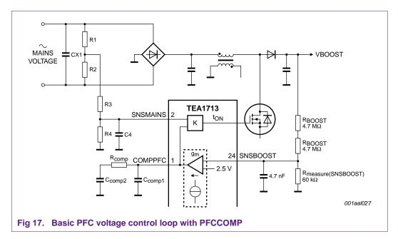
The transfer function has a pole at 0 Hz, a zero by  $R_{comp}/C_{comp2}$  and a pole again by  $C_{comp1}/C_{comp2}$ . Set the zero frequency to 10 Hz while the next pole frequency is at 40 Hz. The zero point and pole frequencies of the compensation network can be calculated as follows:
