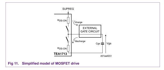
It can be seen from Figure 11 that current is taken from SUPREG when the external MOSFET is switched on by charging the gate to a high voltage.
