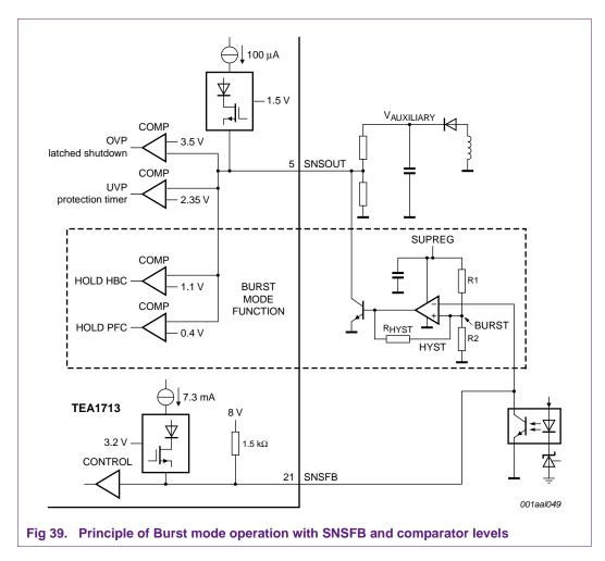
The comparator input monitors the regulation voltage SNSFB to a preset burst voltage value by R1 and R2: BURST. When the HBC power output power is low, the regulation voltage decreases and when it reaches BURST the switching stops by switching SNSOUT to ground. When the switching stops, no energy is converted and the output voltage drops. The regulation voltage then increases again. When the regulation voltage reaches BURST + HYST (voltage hysteresis set by  $R_{HYST}$ ) the switching resumes.
