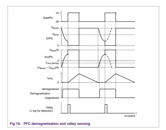
SNSAUXPFC detects the valleys. An auxiliary winding on the PFC coil provides a measurement signal on SNSAUXPFC. It gives a reduced and inverted copy of the MOSFET drain voltage. When a valley of the drain voltage (top at SNSAUXPFC voltage) is detected, the MOSFET is switched on.
