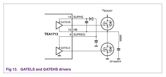
Both HBC drivers have a strong current source capability and an extra strong current sink capability. In general operation of the HBC, fast switch-on of the external MOSFET is not critical, as the HB node swings automatically to the correct state after switch-off. Fast switch off however, is important to limit switching losses and prevent delay especially at high frequency.
