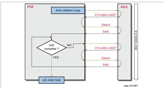
1. The CT (= Cascade Tag, Type A) byte indicates that the UID is not received completely yet. It indicates that another anti-collision loop on the next higher cascade level is required to get the complete UID.
