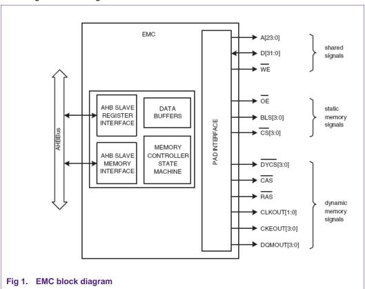
To control a SDRAM memory, the EMC provides the following possible features:
