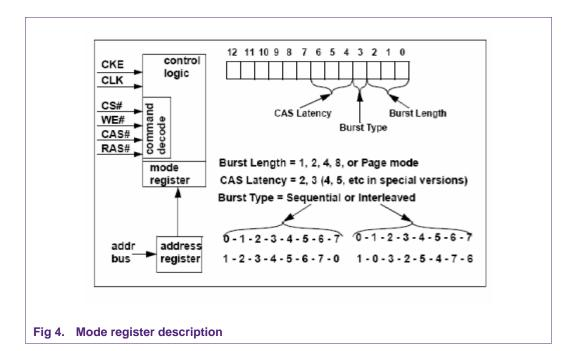
CAS Latency, CL, is the delay, in clock cycles, between the registration of a READ command and the availability of the first piece of output data. The latency can be set to two or three clocks.
