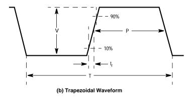
Figure 1. Nomogram of a Trapezoidal Waveform
