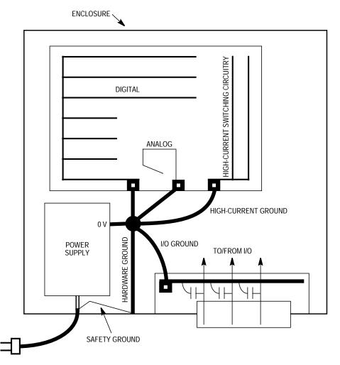
**Figure 4. Typical MCU Application Grounding Example**
