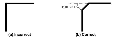
Figure 7. Incorrect (a) and Correct (b) PCB Track Layout for HCMOS Designs
