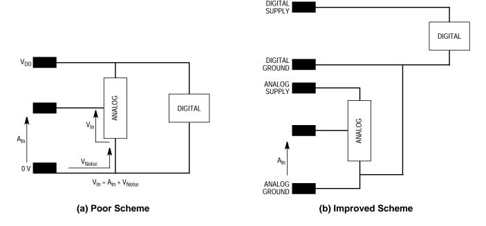
Figure 5. Analog Circuit Grounding
