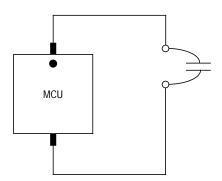
(a) Poor Supply Decoupling
