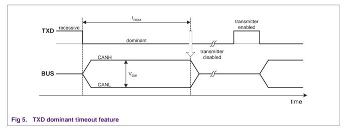
The function of the TXD dominant timeout is illustrated in <u>Figure 5</u>. After a maximum allowed TXD dominant time, the transmitter is disabled. The next dominant output drive is possible only after releasing TXD.
