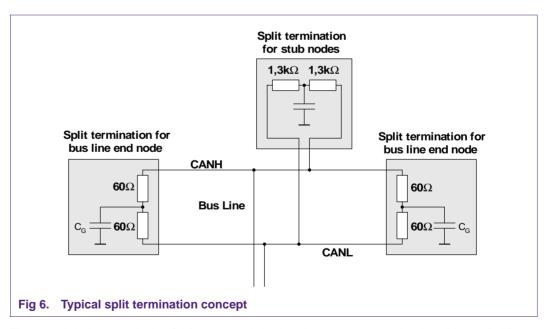
The special characteristic of this approach is that the common mode signal is available at the centre tap of the termination. This common mode signal is terminated to ground via a capacitor  $C_G$  of e.g. 10 nF to 100 nF. However, it is obvious that the capacitor should be connected to a "quiet" ground level. For example a separate ground lead to the ground pin of the module connector with lowest inductance is recommended, if termination is placed inside the bus nodes.
