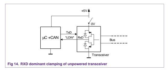
Normally, transceivers are pulling RXD to GND if unpowered, thus clamping RXD to dominant level. This will be recognised by the CAN-controller as a continuous wake-up signal. So it is not possible to put the CAN-controller into its Standby mode when the transceiver is unpowered.
