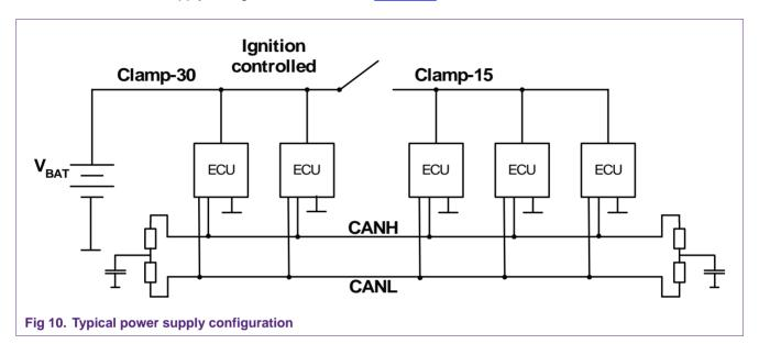
The above mentioned partial networking concept requires that unpowered clamp-15 transceivers must not degrade the system performance. Reverse currents flowing from the bus into unpowered transceivers have to be as low as possible. The TJA1050 is optimised with respect to low reverse currents and is designed for clamp-15 nodes.
