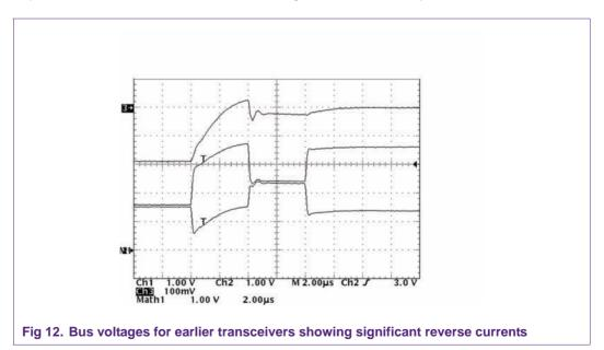
The effect of asymmetrical biasing of the common mode voltage becomes more visible, the more unpowered nodes are present within the system (larger total reverse currents). If there is a large number of unpowered nodes, it is recommended to additionally stabilize the nominal common mode voltage of  $V_{CC}/2$  with an external biasing circuit in order to achieve an optimum EMC performance. Figure 13 illustrates the external biasing circuit,
