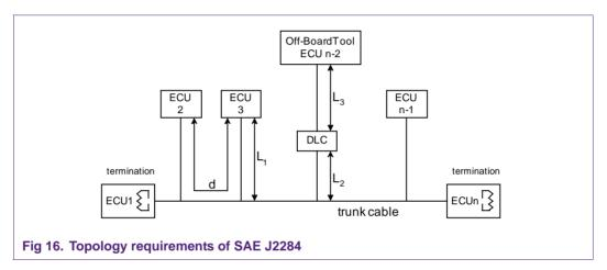
In practice some deviation from the stringent topology proposals might be necessary, because longer stub lengths are needed. Essentially the maximum allowable stub length depends on the bit timing parameters, the trunk cable length and the accumulated drop cable length. For a rule of thumb calculation of the maximum allowable stub length refer to Ref. 7.
