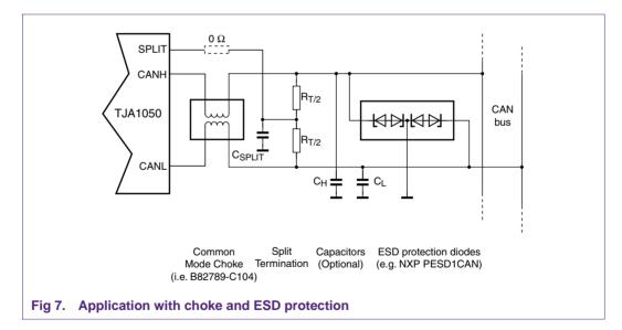
There is always a disadvantage with common mode chokes. The inductance of the choke may establish a resonant circuit together with pin capacitances. This can result in unwanted oscillations between the bus pins and the choke, both for differential and common mode signals. Oscillations of the differential signal can cause multiple switching of RXD.
