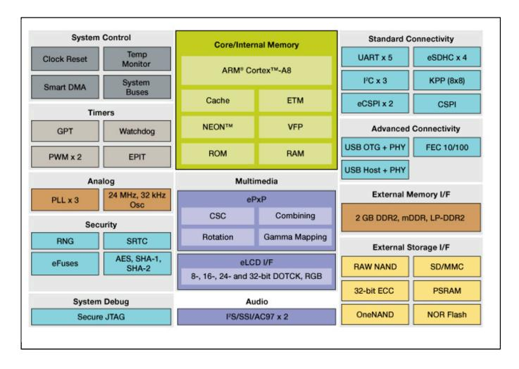
View additional information for Multimedia Applications Processors - LCD Controller, Arm® Cortex®-A8 Core.
