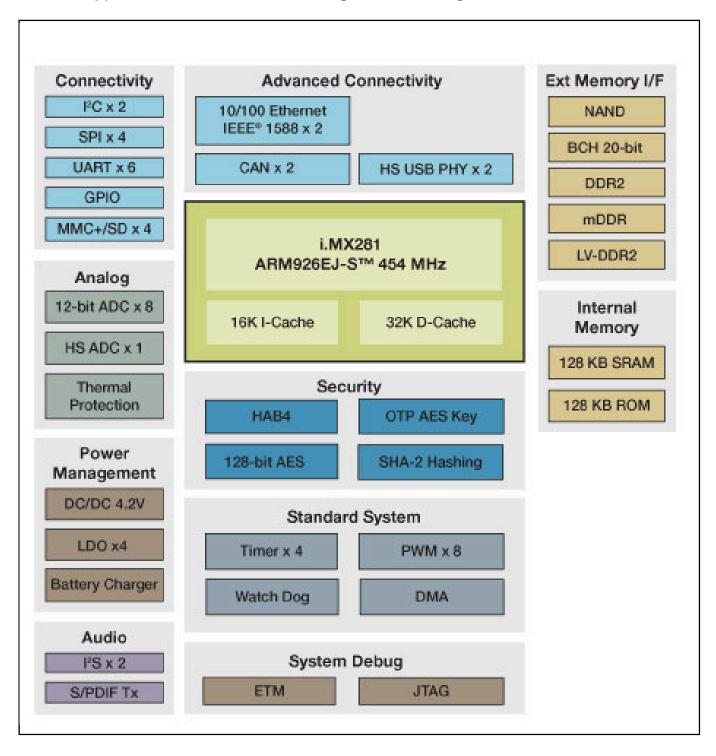
View additional information for Multimedia Applications Processors - Automotive Applications, Connectivity, Integration, ARM9™ Core.
