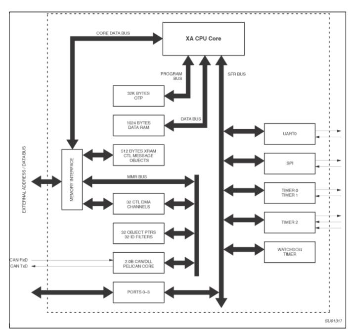
View additional information for XA 16-Bit Microcontroller Family 32K/1024 OTP/ROM CAN Transport Layer Controller 1 UART, 1 SPI Port, CAN 2.0 B, 32 CAN ID Filters, Transport Layer Co-Processor.
