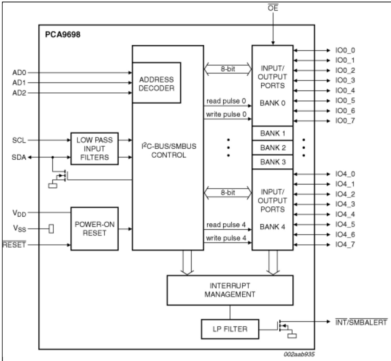
View additional information for [带有RESET、OE和INT的40位Fm+ I<sup>2</sup>C总线高级I/O端口](#).
