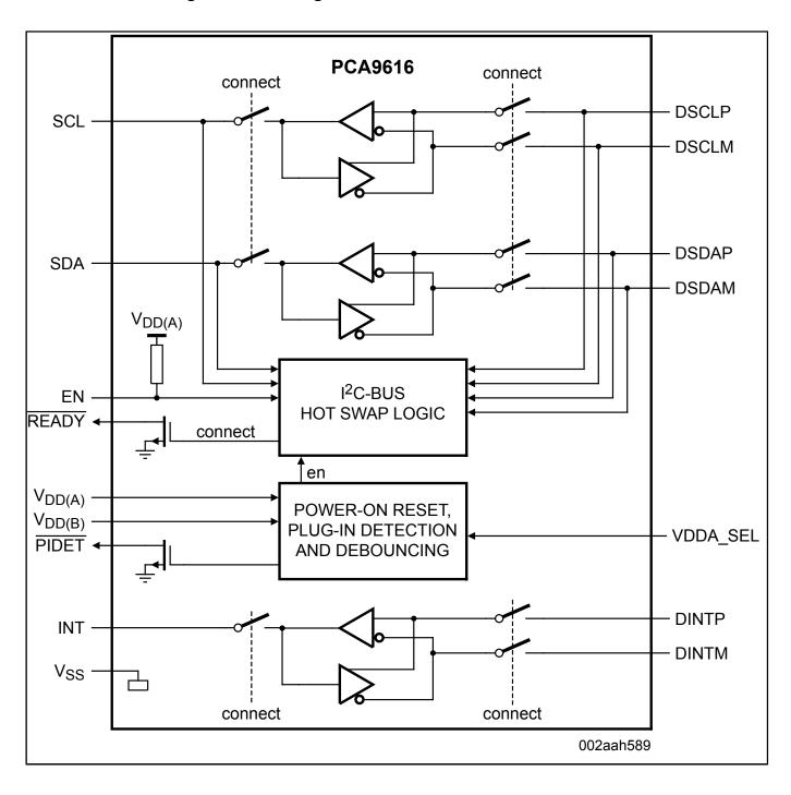
PCA9616 Block Diagram Block Diagram
