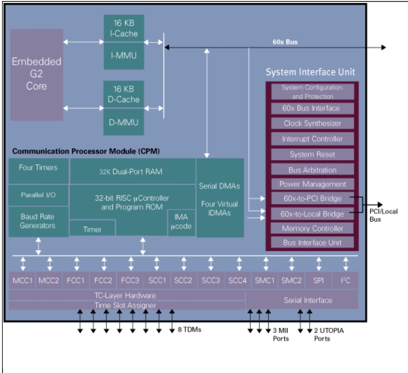
View additional information for PowerQUICC® II处理器带PCI、256个通道。HDLC, UTOPIA II, 10/100以太网, IMA.
