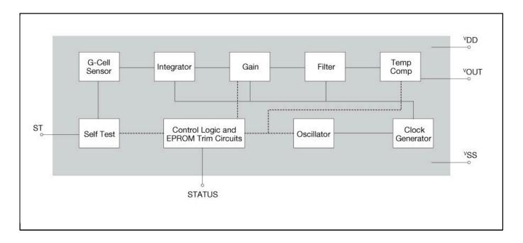
View additional information for  $\pm 7 \mathrm{g}$ ,低重力加速度,模拟加速度传感器.
