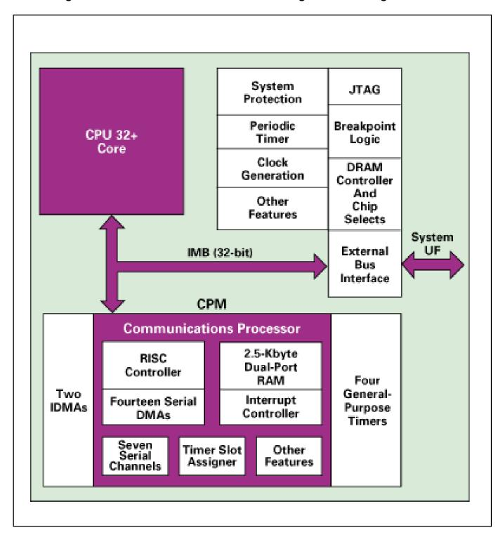
View additional information for Quad Integrated Communication Controller (QUICC).
